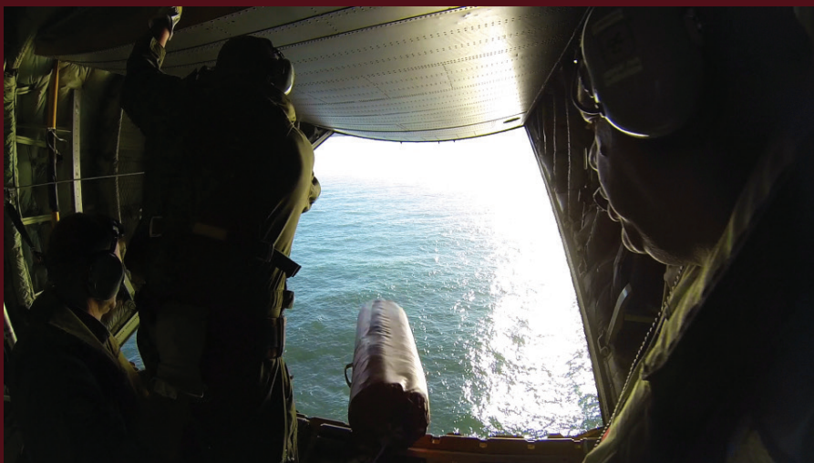
A life raft is pushed out of the back of the aircraft with a small parachute
